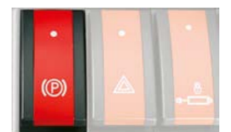
The toggle switch allows the parking brake to be operated manually.
