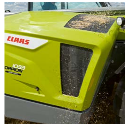
Avoidance of radiator soiling thanks to the reversible fan.
