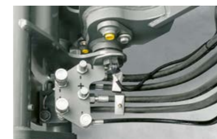
Well-protected hydraulic connections on the implement carrier.
