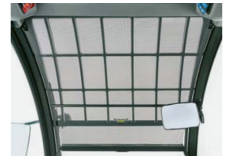
The roof window is fitted with a roll-up sun screen as standard.
