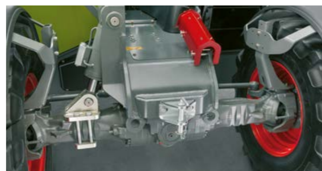
Greater off-road safety thanks to hydraulic levelling.
